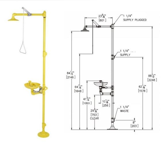
Model S1320 is our combined safety shower and eye wash with plastic head and bowl. Complete with yellow plastic spray heads and bowl and plastic shower head. Supplied with a 1" chrome plated brass stay open ball valve with stainless steel pull handle and activation lever for the shower and a 1/2" chrome plated stay open ball valve and stainless steel push handle for the eye wash.
